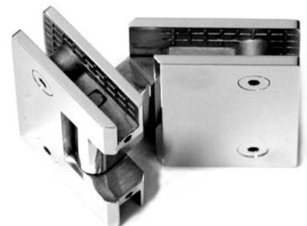
#85.109 ; 135 degree glass hinge for 10 to 12 mm -3/8 to 1/2 inch glass; leaf: 89 x 61 x 65 mm; (3 1/2 x 2 3/8 x 2 1/2 inch)
