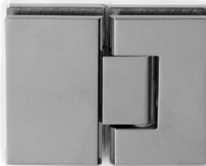
#85.121 ; Flush glass hinge for 10 to 12 mm -3/8 to 1/2 inch glass; leaf: 89 x 54.6 mm; (3 1/2 x 2 1/8 inch) total length 112 mm (4 inch)
